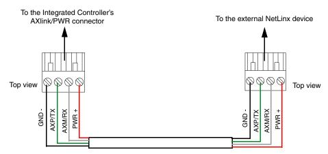
FIG. 8 Mini-Phoenix connector wiring diagram (direct data and power)
